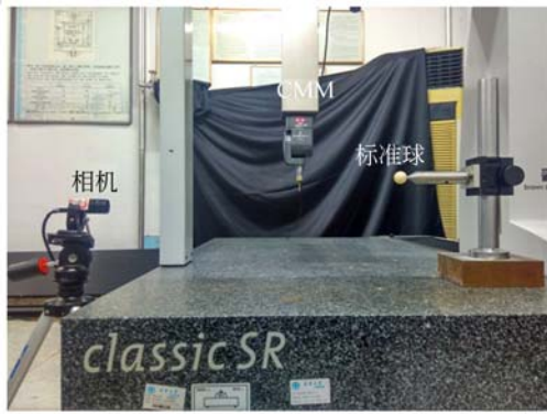
图 8 相机和三坐标测量机位姿关系标定系统示意图 Fig. 8 Schematic diagram of calibration system for altitude relation between camera and CMM
