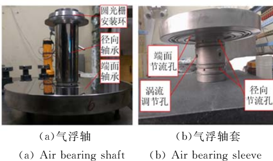
图 8 气浮轴及气浮轴套实物 Fig. 8 Photograph of air bearing shaft and sleeve
