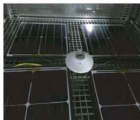
(b) 老化试验样品接线图 (b) Sample wiring of aging test
