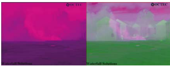
(a)Waxman 融合图像 (b)本文融合图像 (a)Waxman fusion image (b)Fusion image by proposed method
