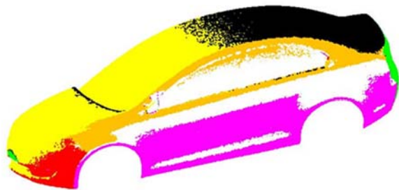
(a) 基于 FCM 聚类的分割 (a) Segmentation based on FCM clustering
