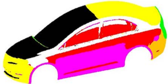
(b) 基于遗传的 FCM 聚类的分割 (b) Segmentation of FCM clustering based on genetic algorithm
