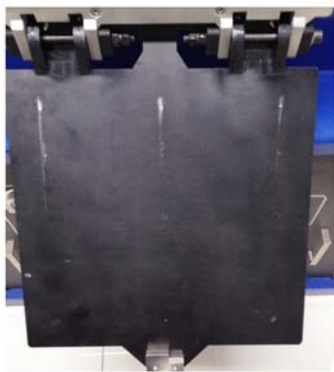
图9 舱门与立方星接触痕迹
