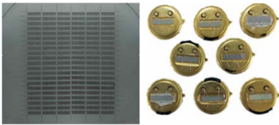
(a) SAW 传感器阵列 (b) 封装后的 SAW 传感器 (a) Arrays of SAW sensors (b) Packaged SAW sensors
