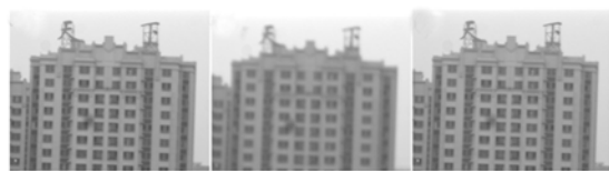
(a) 温度变化前 (b) 温度变化后 (c) 调焦补偿后 (a)Before temperat- (b)After temperature (c)After focusing ure changed changed compensation
