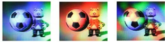
(b) 视场角左边界以外、视场角以内和右边界以外的像 (b) Image outside the left boarder, image inside and the one outside right boarder of viewing angle
