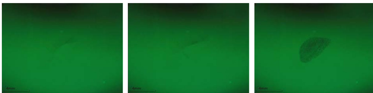
(a)能量密度为 7.96 J/cm 2 附近时的显微图 (b)能量密度为 10.75 J/cm 2 附近时的显微图 (c)能量密度为 15.13 J/cm 2 附近时的显微图 (a)Micrograph of area with energy density of 7.96 J/cm 2 (b)Micrograph of area with energy density of 10.75 J/cm 2 (c) Micrograph of area with energy density of 15.13 J/cm 2
