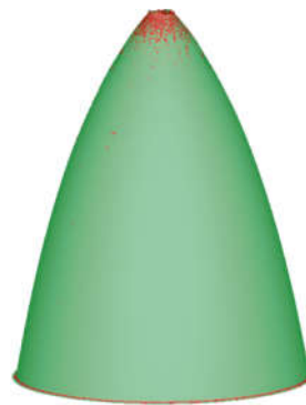
图 4 非可靠点筛选结果(红色点) Fig. 4 Filtering result of unreliable points (in red)
