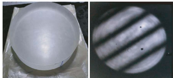
(a) 粗糙表面光学元件 (b) 光学元件的干涉图像 (a) Optical component with rough surface (b) Fringe image of optical component
