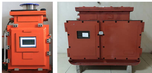
图 6 两种形式隔爆仪器安装外壳 Fig. 6 Two forms of flameproof enclosure
