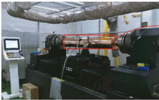
(a) 辊筒模具超精密机床 (a) Drum roll lathe
