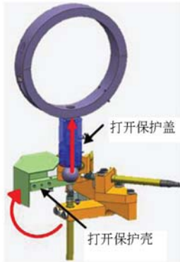
(a) 在测量配置中打开保护盖和保护壳的测量装置 (a) A measuring device that opens a protective cover and a protective shell in the measurement configuration
