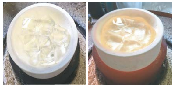
(a)玻璃表层塌陷 (a) Surface of glass was collapsed (b)迅速熔化 (b) Melts rapidly
