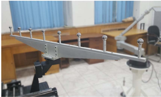
图 4 包含 8 个直径已知的球体 (相邻球体间距 200 mm)的球杆 Fig. 4 Pre-measured ball bar with 8 spheres that equally spaced at intended 200 mm intervals
