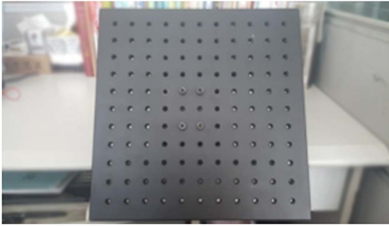
图 3 用于单点锥窝实验(SPAT)的洞板 Fig. 3 Conical hole plate for single-point articulation performance test (SPAT)
