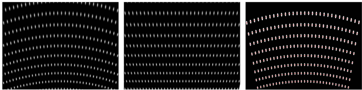
(a)基于高斯结构光的曲面采集图像 (b)基于高斯结构光的平面采集图像 (c)曲面采集图像预处理 (a)CPAI based Gauss structured light (b)PAI based Gauss structured light (c)CPAI preprocessing
