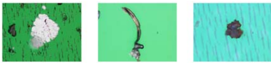
(a)疲劳磨粒 (b)切削磨粒 (c)氧化物磨粒 (a)Fatigue debris (b)Cutting debris (c)Oxidative debris
