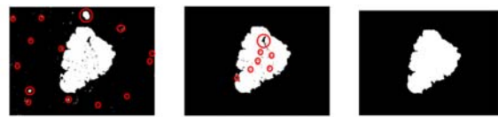
(a)二值化图像 (b)外部滤波 (c)滤波结果 (a) Binary image (b)External filtering (c) Filtering result
