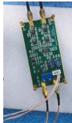
(b)正交解调模块 (b)Quadrature demodulation module
