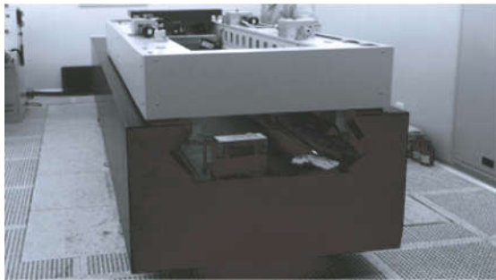
(a) 自行研制的弯月面大尺寸涂胶设备 (a) Meniscus-base coating device with the big area
