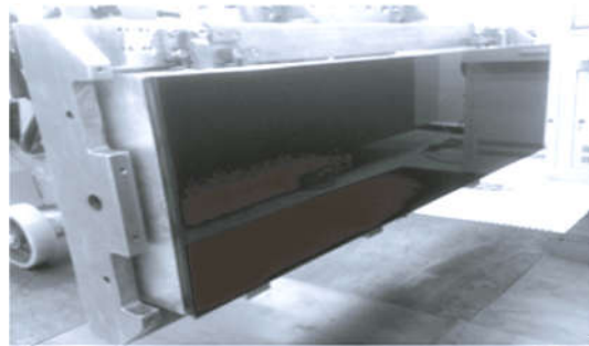
(b) 基于弯月面调控涂胶实现的大尺寸涂胶基片 (b) Big area substrate coated by meniscus-controlling
