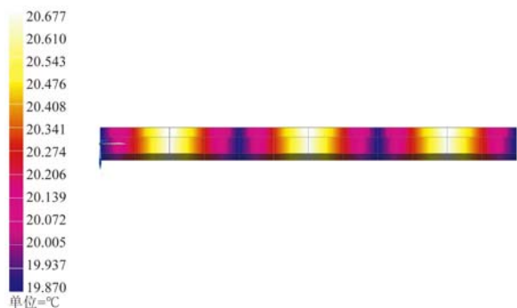
图 6 等效热导率为 41.3 W/(m·K) 的单根桁架杆温度分布 Fig. 6 Temperature distribution of single truss with equivalent thermal conductivity of 41.3 W/(m·K)
