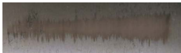
(a) CAM 软件规划姿态抛磨 (a) Grinding with CAM software planning posture
