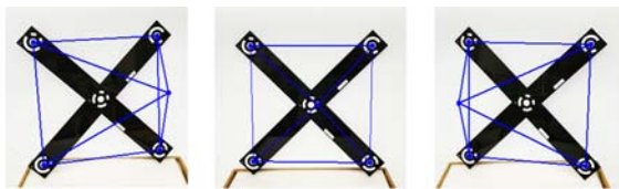
(c) 本文目标函数虚拟长方锥体的重投影结果 (c) Re-projection results of virtual rectangular pyramid based on proposed objective function
