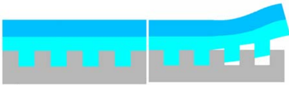
(a)三层结构示意图 (b)脱模过程示意图 (a)Schematic diagram of three-layer structures (b)Schematic diagram of demolding process
