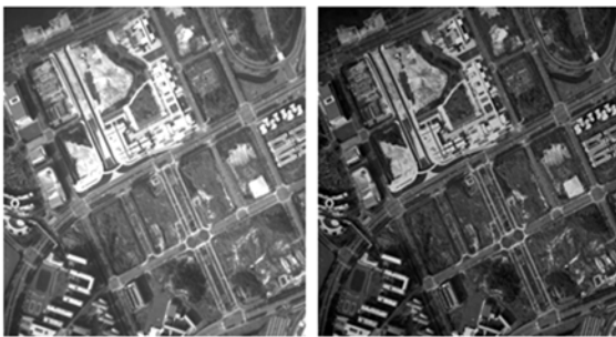
图 8 真实降质图像‘city’(左)及 SDIWF-IBD 复原结果(右) Fig. 8 Real degraded image ‘city’(left) and restoration result by SDIWF-IBD(right)
