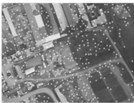
(a) 尺度因子为 \sigma=1.5 时, Harris 检测器检测的角点 (a) Corners detected by Harris in \sigma=1.5
