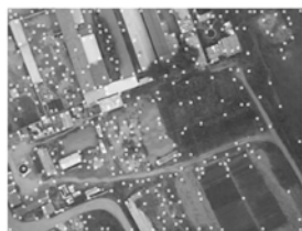
(b) 尺度因子为 \sigma=1.5 时, 基于优化梯度滤波 Harris 检测器检测的角点 (b) Corners detected by optimal derivative filters based Harris in \sigma=1.5
