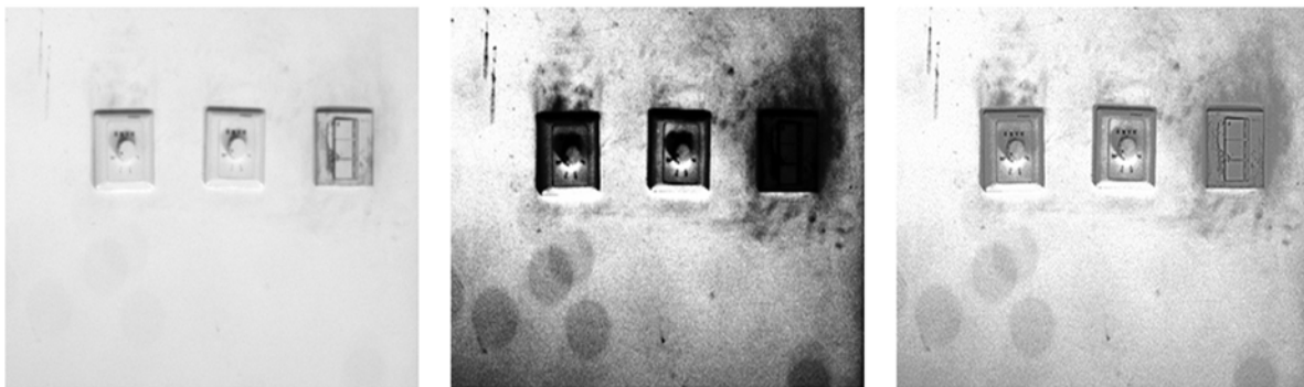
(a)原图 (b)直方图均衡化结果 (c)本文算法增强结果 (a)Original image (b)Histogram equalization result (c)Enhancement result by proposed algorithm
