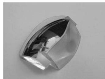
图 6 采用回转对称的非球面面型的曲面棱镜 Fig. 6 Photo of prism with aspheric surfaces
