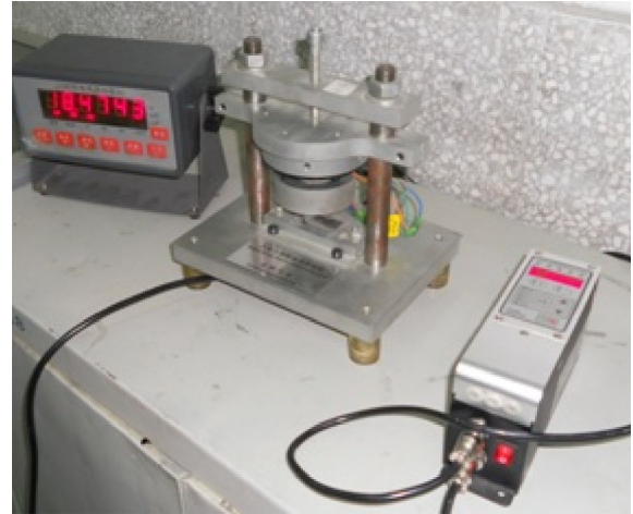
图 3 作用在试件上的动载荷测试实验装置图 Fig. 3 Test devices of dynamic load on the specimen measured by prototype
