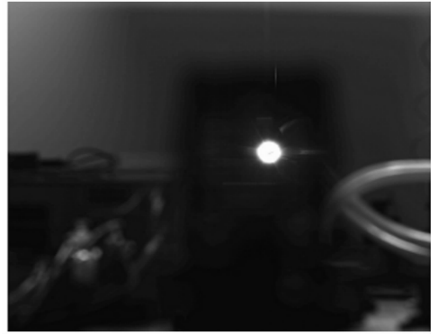
图 3 TDI CCD 在重复脉冲激光辐照下无明显背景条纹的图像 Fig.3 Picture without obvious background fringes from TDI CCD under irradiation of repetitive pulse laser
