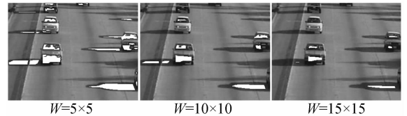
图 3 基于相关比方法在不同窗口大小下的检测效果 Fig. 3 Detection performance obtained by correlation ratio in different window sizes
