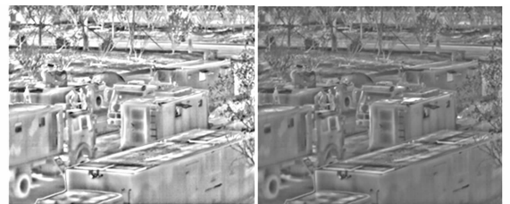
(a)传统方法获取的细节层 (b) GL- \Phi 获取的细节层 (a)Detail layer acquired by traditional method (b) Detail layer acquired by GL- \Phi method
