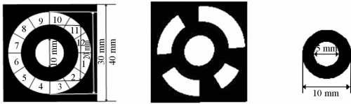
(a) 编码标记点 (b)编码标记点实际成像 (c)非编码标记点 (a)Coded target (b)Imaged coded target (c)Non-coded target
