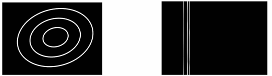
(a) 同心椭圆 (b) 经 ALPC 变换所得平行直线 (a) Concentric ellipses (b) Parallel lines after ALPC
