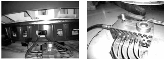
(a)方位轴基座 (b)齿轮分油器 (a)Basement of azimuth (b)Gear oil separator
