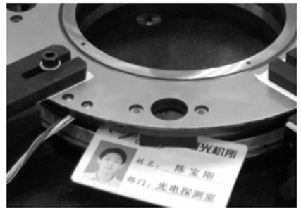
图 9 读数头与光栅间隙达到 2 mm Fig. 9 Gap between reading head and grating is about 2 mm
