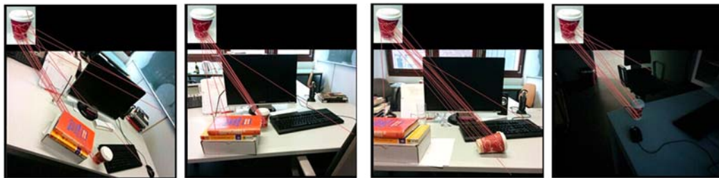
(a) 原 SIFT 算法视角变化情况下目标识别效果 (b) 原 SIFT 算法局部遮挡情况下的目标识别效果 (c) 原 SIFT 算法目标旋转情况下的目标识别效果 (d) 原 SIFT 算法弱光照情况下的目标识别效果 (a) Recognition results by using original SIFT in viewpoint change condition (b) Recognition results by using original SIFT in external occlusion condition (c) Recognition results by using original SIFT in object rotation condition (d) Recognition results by using original SIFT in weak illumination condition
