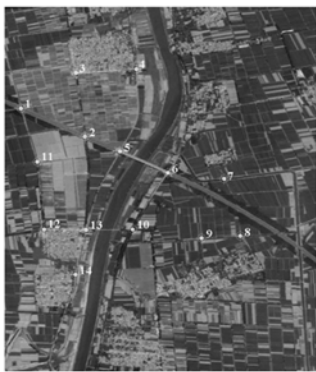
(a) SPOT6 提供的参考正射投影图像(14 个检验点) (a) Reference orthoimage from SPOT6 satellite (14 checkpoints)
