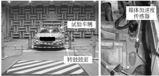
(a) 实车转鼓试验 (b) 传感器位置示意 (a) Full vehicle test on the chassis dynamometer (b) Sensor layout
