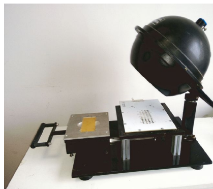
图 3 LED 测试机械结构 Fig. 3 Mechanism of LED measurement
