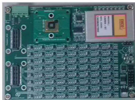
图 12 APD 阵列信号采集模块实物图 Fig.12 Picture of signal sampling module for APD array
