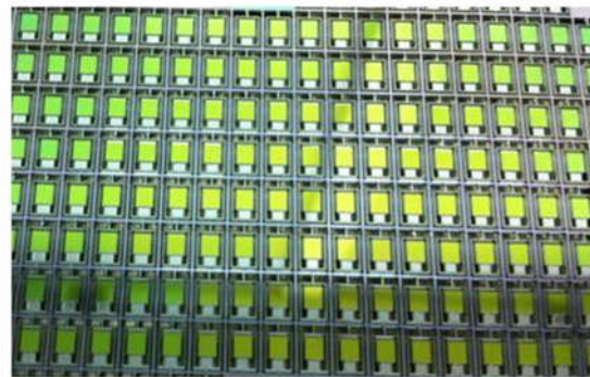
(a) 硅基悬臂梁-质量块结构阵列 (a) Fabricated silicon wafer with arrayed spring-mass unit
