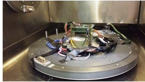
图 3 MEMS陀螺及恒温实验设备 Fig. 3 MEMS gyro and its test device
