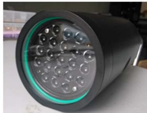
图1 小型化光学隐蔽深度测量系统的21个测量通道 Fig.1 Twenty-one measurement channels of miniaturized optical concealment depth measuring system
