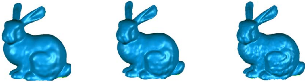
(a) Laplace 迭代 5 次去噪结果 (b) 双边滤波迭代 2 次的去噪结果 (c) 本文算法迭代 2 次的去噪结果 (a) Denoising results of Laplace with 5 times of iterations (b) Denoising results of bilateral filter with 2 times of iterations (c) Denoising results of proposed method with 2 times of iterations
