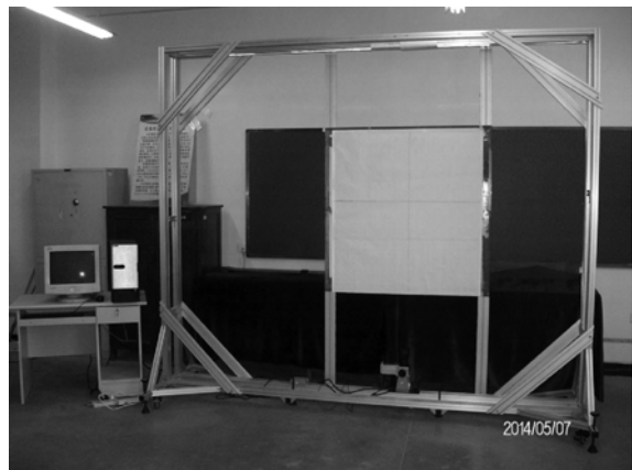
图 9 单线阵 CCD 立靶系统实物照片 Fig. 9 Physical photos for single linear CCD camera for simulation of dual-target measurement system
