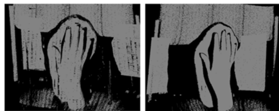
(c)未经过滤波后的重构图 (c)3D reconstruction result without global phase filter (d)全局相位滤波后重构图 (d)3D reconstruction result after global phase filter
