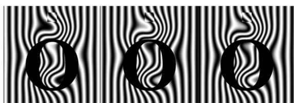
图 4 三幅经过物体高度调制的相移光栅 I_1 , I_2 和 I_3 Fig. 4 Gratings I_1 , I_2 and I_3 which are modulated by the objects
