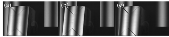
图 8 (a)~(c)光栅采集图 Fig. 8 (a)-(c) The phase-shifted patterns
