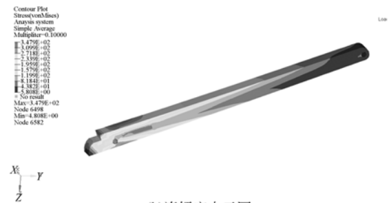
(b)连杆应力云图 (b)Stress contour of rod
