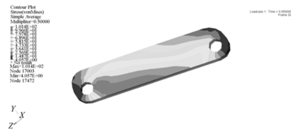
(a)耳片应力云图 (a)Stress contour of lug
