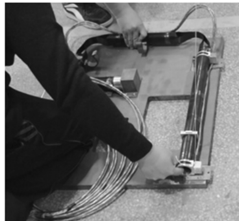
(a) 碳纤维伸杆收拢 (a) Carbon fiber boom folded
