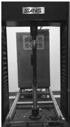
(a) 碳纤维伸杆拉伸过程 (a) Carbon fiber boom stretching process
